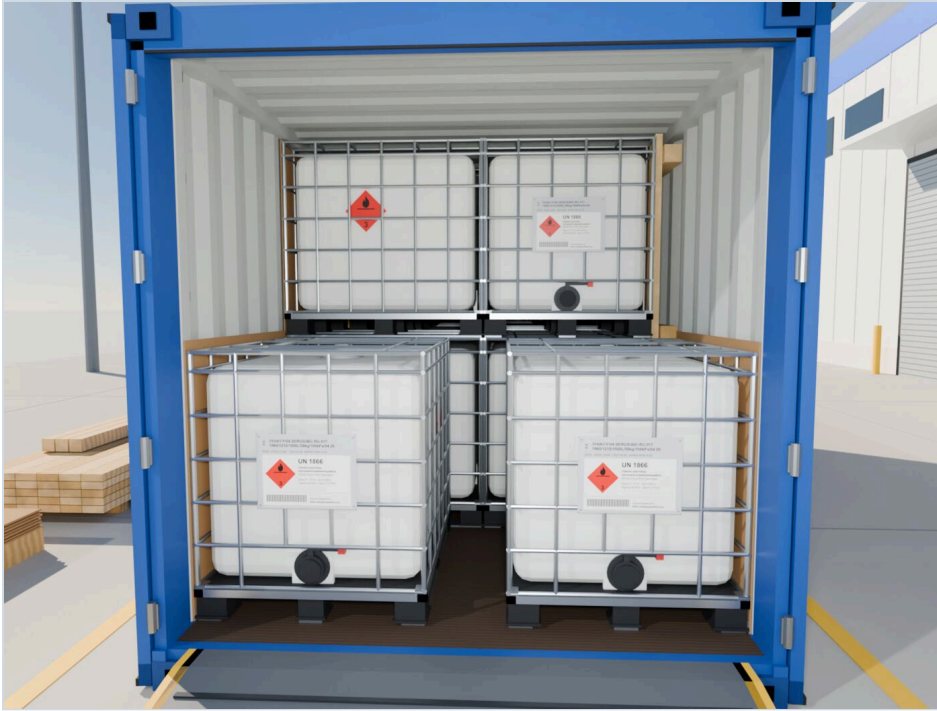
STAGE PHOTO 09 Fifth row: 2 totes against the side walls, cardboard at the sides — door opening without the shield
