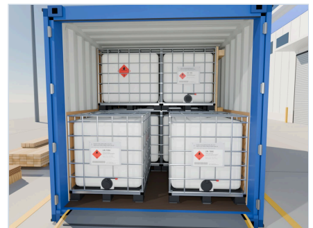
09 Fifth row: 2 totes against the side walls, cardboard at the sides — door opening without the shield
