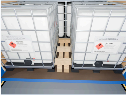
10 Stop structure between the fifth-row totes: 100×100 stop and middle bars
