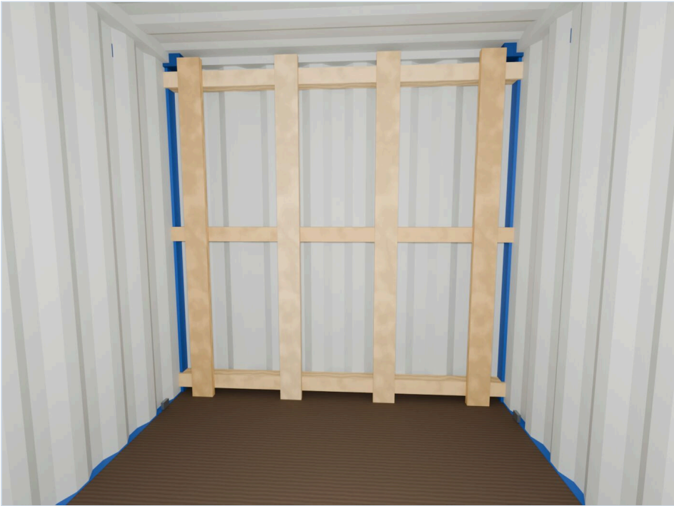
STAGE PHOTO 04 End wall shield: 3 bars 100×100 against the wall, ends in the corrugations, 4 vertical boards on top
