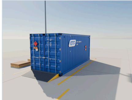
14 Container closed, 250×250 mm hazard placards on all four sides
