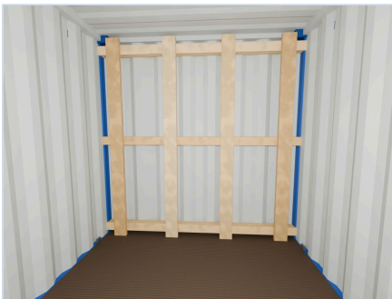
04 End wall shield: 3 bars 100×100 against the wall, ends in the corrugations, 4 vertical boards on top
