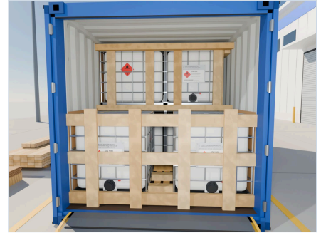
12 Door opening with the shield
