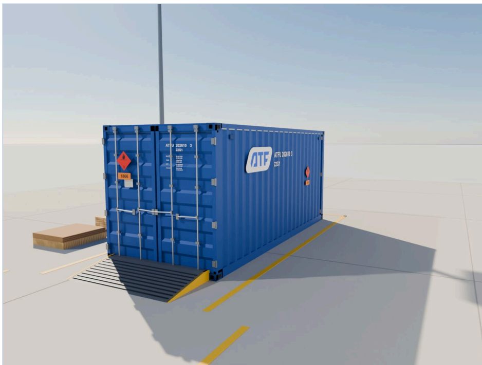
STAGE PHOTO 13 Container closed, 250×250 mm hazard placards on all four sides
