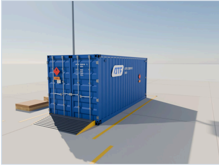
13 Container closed, 250×250 mm hazard placards on all four sides
