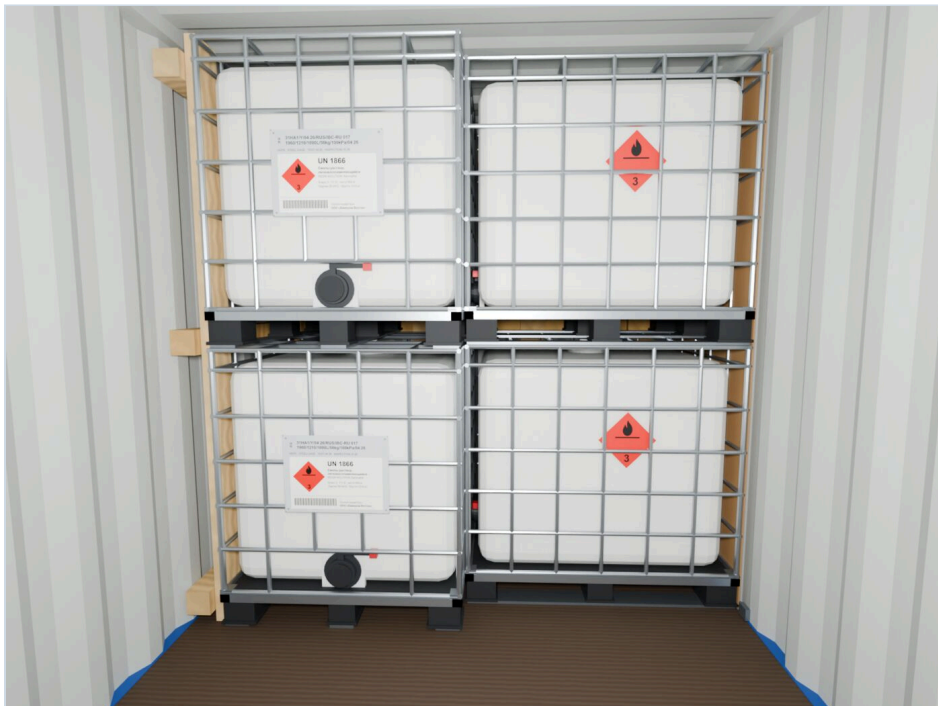
STAGE PHOTO 05 First full row from the end wall
