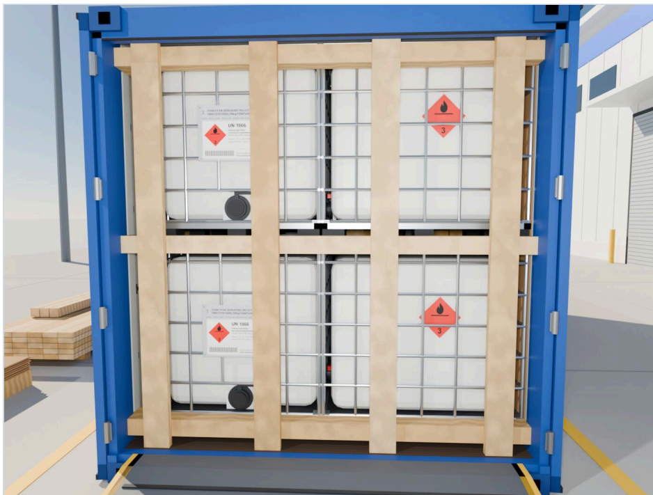
STAGE PHOTO 11 Door opening with the shield
