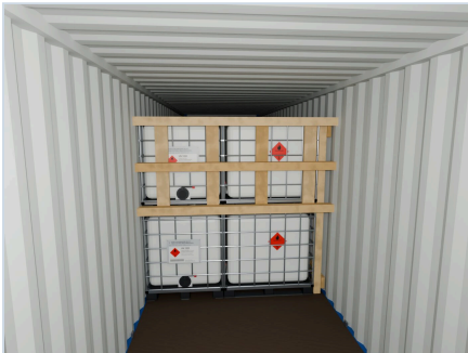
13 Second-tier shield on the door side
