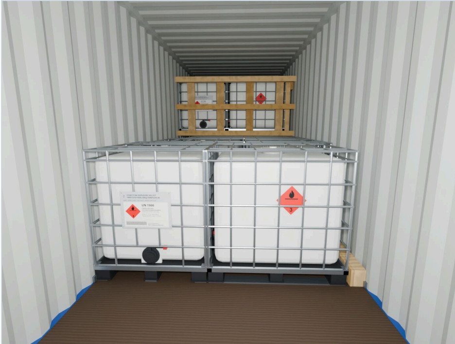
STAGE PHOTO 16 Row 8: units 19 and 20, bar pos. 7 at the right wall
