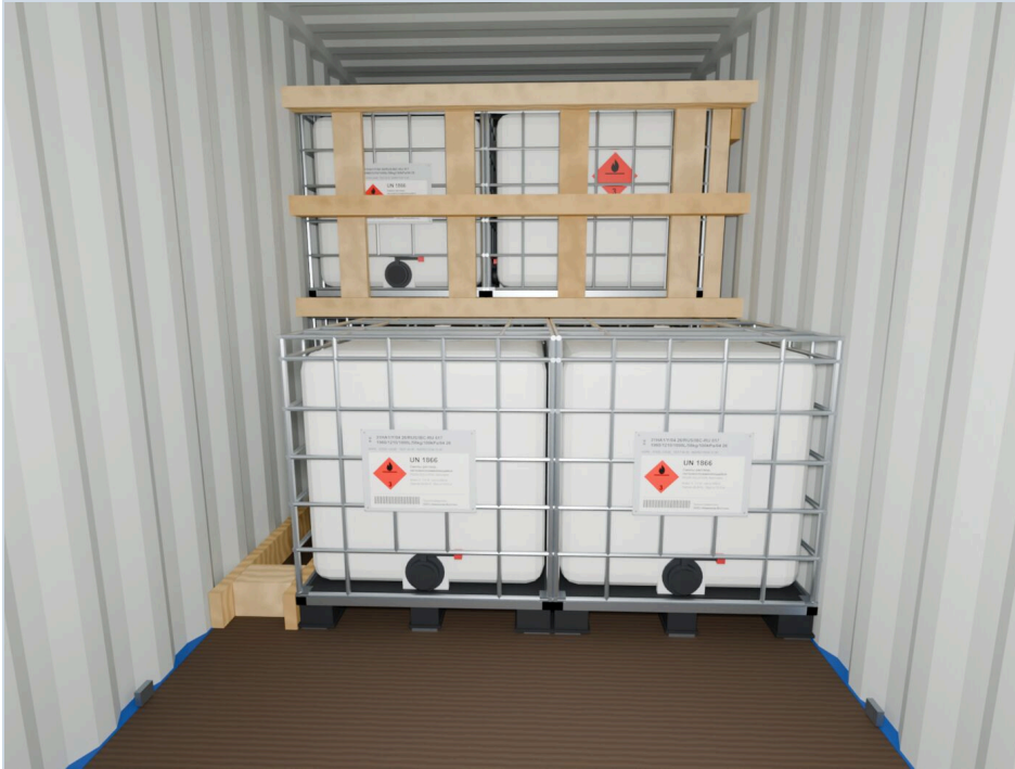
STAGE PHOTO 14 Row 6: units 15 and 16, stop structure at the left wall
