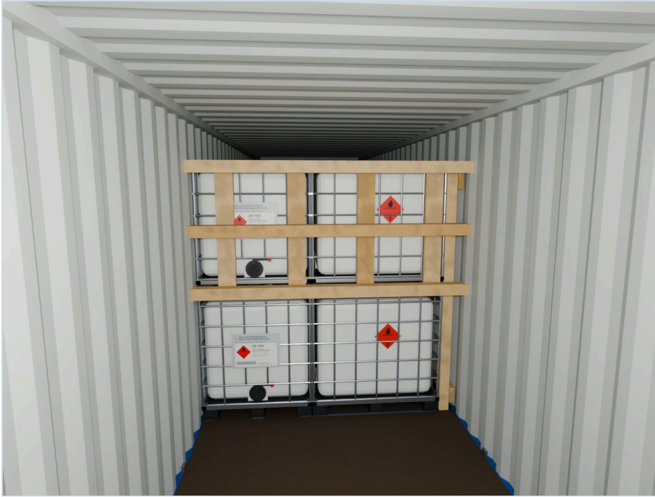
STAGE PHOTO 13 Second-tier shield on the door side
