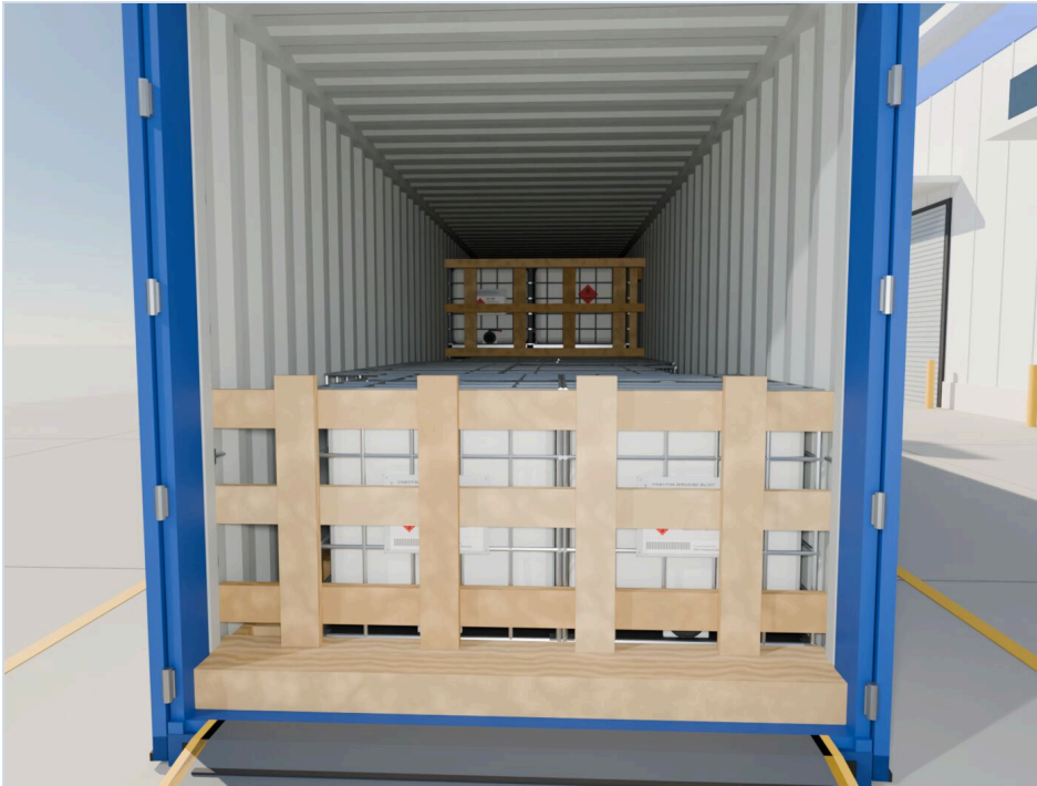
STAGE PHOTO 19 Door opening with the shield and stop bars pos. 1
