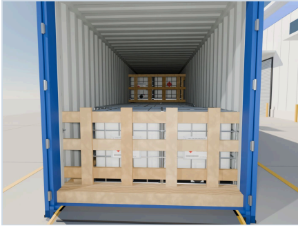
19 Door opening with the shield and stop bars pos. 1
