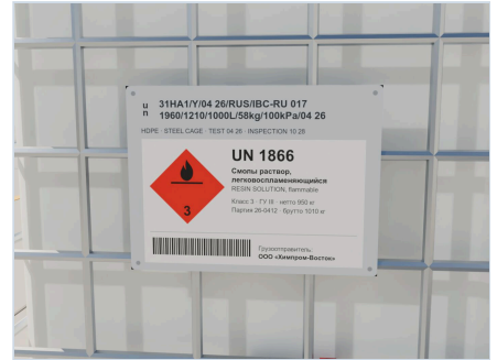
03 Packaging marking close-up — every character legible The tote plate close up, straight on, without glare: every character of the marking is legible.
