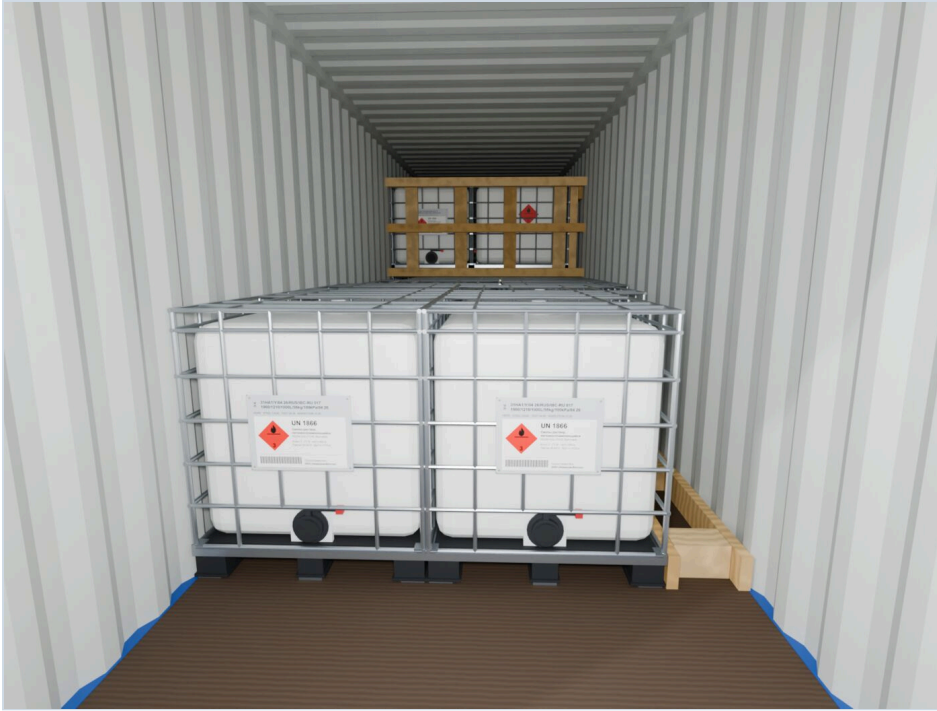
STAGE PHOTO 17 Row 9: units 21 and 22, stop structure at the right wall
