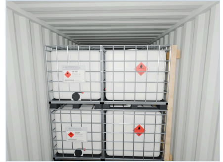
12 Row 5, second tier: units 13 and 14, shield at the right wall
