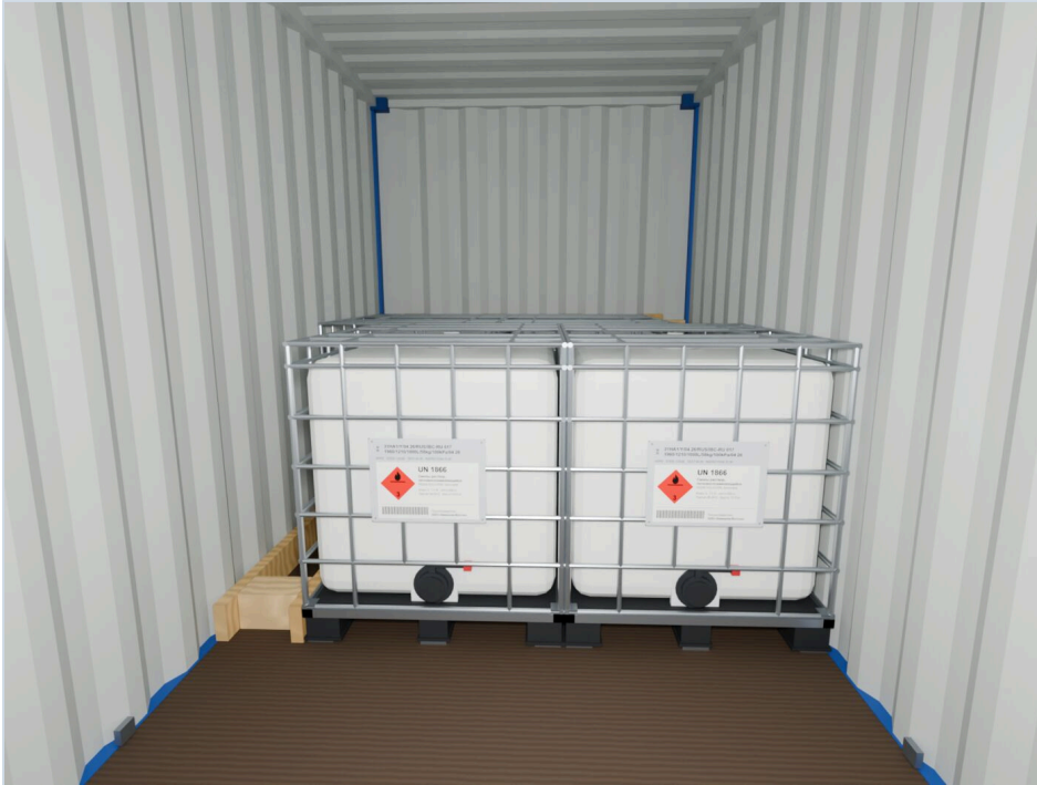
STAGE PHOTO 06 Row 2: units 3 and 4, stop structure at the left wall
