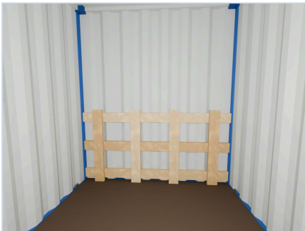
04 End wall shield: 3 horizontal boards pos. 4 at the wall, 4 vertical boards pos. 3 From inside the container towards the end wall, 2–3 m away: the whole shield, ends of the horizontal boards in the corrugations.
