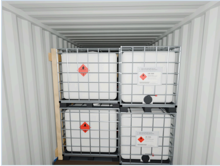
10 Row 4, second tier: units 9 and 10, shield at the left wall
