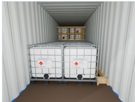
17 Row 9: units 21 and 22, stop structure at the right wall
