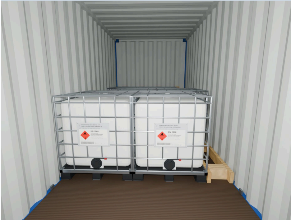
STAGE PHOTO 07 Row 3: units 5 and 6, stop structure at the right wall
