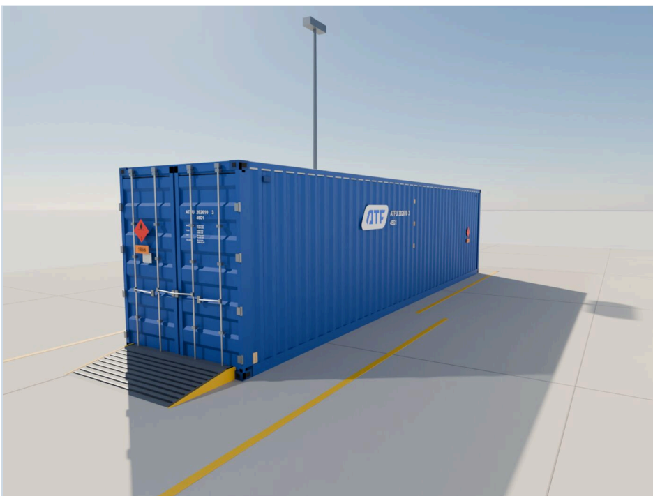
STAGE PHOTO 21 Container closed, hazard placards on all four sides (for dangerous goods)
