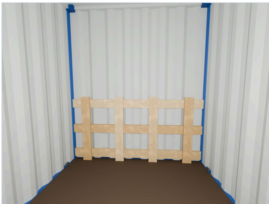
STAGE PHOTO 04 End wall shield: 3 horizontal boards pos. 4 at the wall, 4 vertical boards pos. 3
