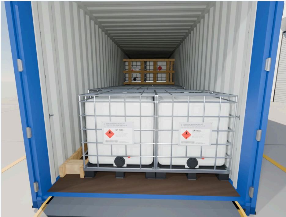
STAGE PHOTO 18 Row 10: units 23 and 24 — door opening without the shield
